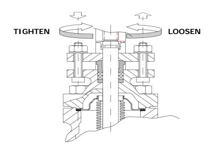
□ Leaks between the body and bonnet: Possibly the gasket between these two elements (Figures GV-116 GV-340) or between the hood and the body (Figures BGV-116, BGV-216, BGV-225, BGV -340) has deteriorated. Proceed to its replacement.
