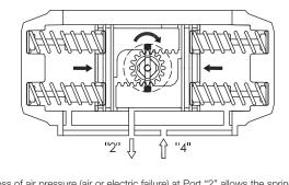
The loss of air pressure (air or electric failure) at Port "2" allows the springs to force the pistons inward. A clockwise rotation is achieved. Exhaust air exits from Port 2.
