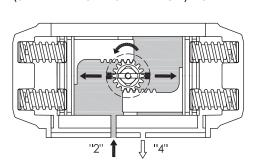
Air supplied to Port "2" forces the pistons toward the actuator end caps, compressing the springs. A counter-clockwise rotation is achieved. Exhaust air exits from Port 4.
