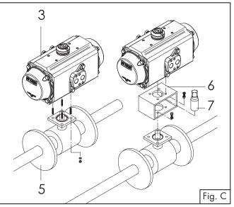
Important: when using a spring return actuator for a fail safe operation, ensure that when air or electricity failure occurs the direction of rotation is correct for your application. Fit the actuator 3 onto the valve 5. It is possible to assemble
