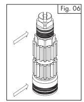
• Insert partially the drive shaft (60) in the body (50), install octi-cam (01) in the correct position (for standard assembly or for lock-out) as shown in figures 07 and 07A, related to the bottom and top of the drive shaft and the rotation of the actuator when energised. Install the internal thrust bearing (08). Insert completely the drive shaft in the body.
