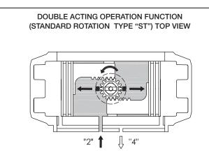
Air supplied to port 2 forces the pistons towards the actuator end caps. A counter-clockwise rotation is achieved. Exhaust air exits from Port 4.
